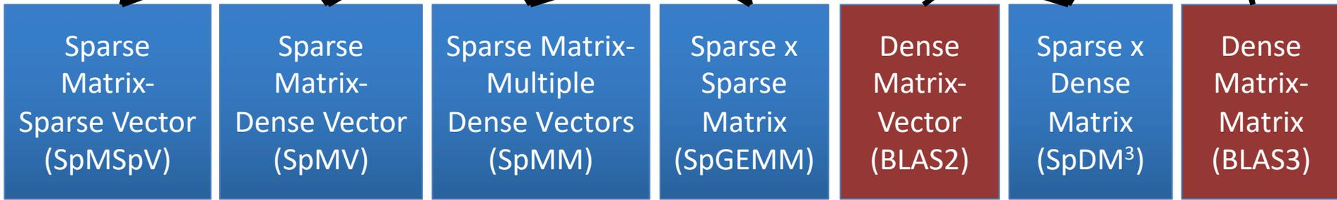
Graph/Sparse/Dense BLAS functions (in increasing arithmetic intensity) →
